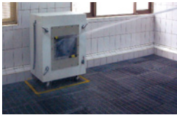
IEI's LCD products are front sealed and tested in the certified house chamber under UL's Witnessed Test Data Program (WTDP).
