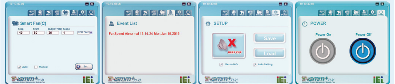
Smart Fan Control Advanced fan setting for both CPU and system smart fan
